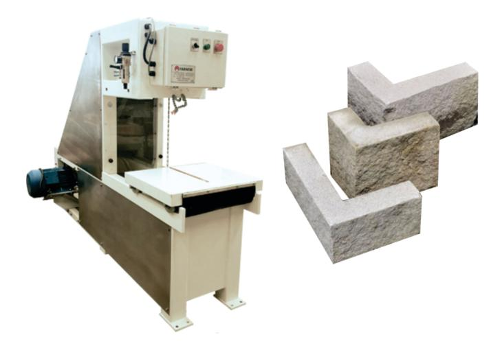
The WIRE SLITTER has been conceived for small block cutting and producing quoins from sandstone.
